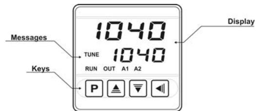
**Figure 02** - Identification of the parts referring to the front panel
