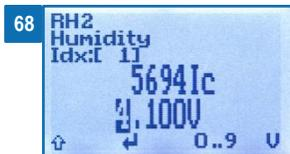
8. Now enter the real humidity value, the temperature, the displayed humidity value and the new Ic value (point 7) of the humidity standard used into the corresponding fields in the MS Excel calculation sheet (figure 69).
