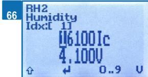
5. Enter the indices 1 to 6 of the Ic values already stored in the device into the corresponding fields of the MS Excel calculation sheet, paying attention to the volt values (figure 67) ein. Navigate through the indices by pressing
