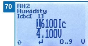
5. Overwrite the current Ic-value with the new calculated Ic-value for this index (figure 71). To do so, press and hold **0..9** to quickly scroll to the required number and either press it for 3 seconds or press
