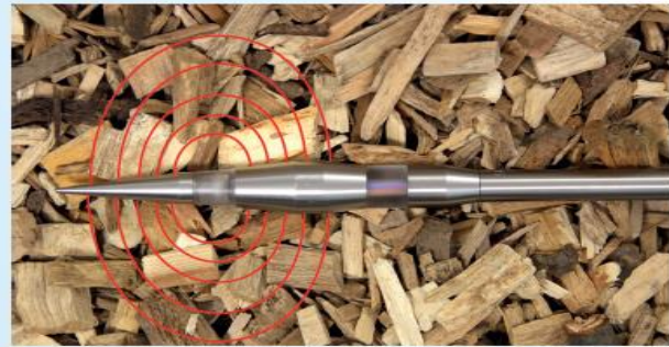
Devices using conductance measurement: BL2, BLL, WLW, BLW, wood chips moisture transmitter,
