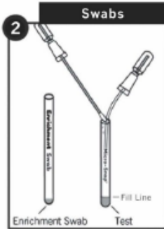
2.1: Swabs: Aseptically transfer 0.1mL (3 drops or to fill line) enriched sample from Incubation Device to Coliform Detection Device.
