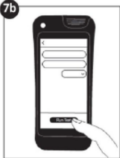
7b. EnSURE™ Touch automatically saves your results. If a positive result is obtained for Coliform, presence of E. coli can be verified using E. coli Detection Device. Repeat measurement procedure above using another aliquot sample from same sample. To get the most value out of your EnSURE™ Touch, register and sync it wirelessly to SureTrend™ Cloud where you can generate meaningful reports and view datasets.
