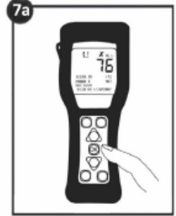
7a. Record RLU results and refer to the Results Interpretation Table for the conversion. If a positive result is obtained for Coliform, presence of E. coli can be verified using E. coli Detection Device. Repeat measurement procedure above using another aliquot sample from same sample.
