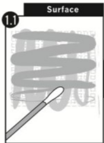
1.1 Surface: Swab 10x10cm area with Enrichment Device.
