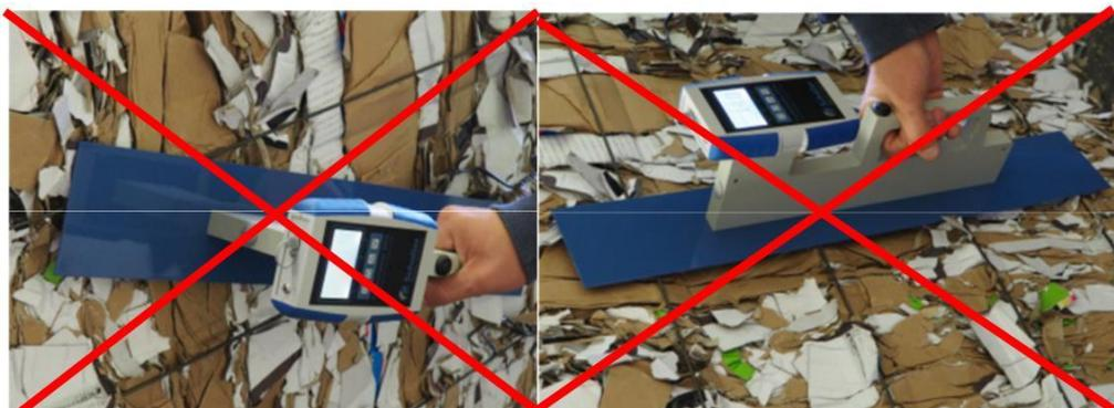
***Connected USB cable during measuring***
