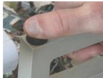
The humimeter RP6 automatically calculates the average moisture content of the saved values. Please avoid measurements at apparently wet areas of the bale, as they do not represent the average moisture content of the bale.
