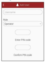
Enter a **Username** for the new user and then select a **Role**. Users can be setup up as Operators or Administrators. Operators perform testing while Administrators manage the instrument and have access to all of the settings.
