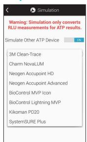
Turning on Simulation Mode converts the RLU results from ATP testing on your EnSURE Touch so that they simulate the results you'd get if you were using another system.
