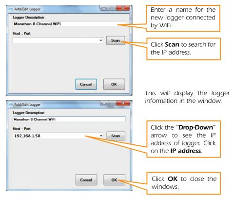
The logger should be connected to the WiFi network and ready for use.
