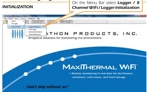
This will open a new window to program the logger's 8 channels.
