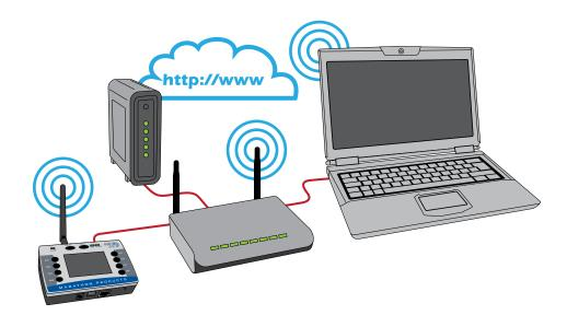
The 8 Channel WiFi logger can connect to your network by either 802.11g WiFi or by standard 10/100 network cable.
