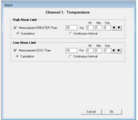
Continuous Interval alarm will trigger if the temperature exceeds the acceptable range for a continuous period of time. E.g. if the Continuous interval option is selected and the time set is five minutes, then the alarm will trigger if five minutes have passed and all of the measurements
