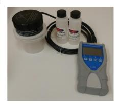
Please note the Aw standards shouldn't be left open. Close the lid immediately when not in use with the Aw measuring unit. Store and use at room temperature and away from sunlight (at +15°C to +25°C)
