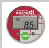
1. REC - 8.6C shows Recording and current temperature
