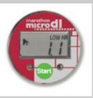
7. LOW HR - 1.1 shows alarm time hours over low threshold
